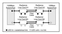
Since the entire main link must appear down if any of its connecting segments fails, the copper ports of line cards A1 and A2 must be able to indicate a no-link condition to their corresponding switch/hubs. To do this, auto-recovery must be enabled on both Radiance line cards A1 and A2
