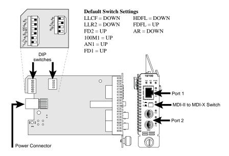
When setting DIP switches,\* the UP position is when the lever of the DIP switch is pushed away from the circuit board. The DOWN position is when the lever is pushed toward the circuit board.
